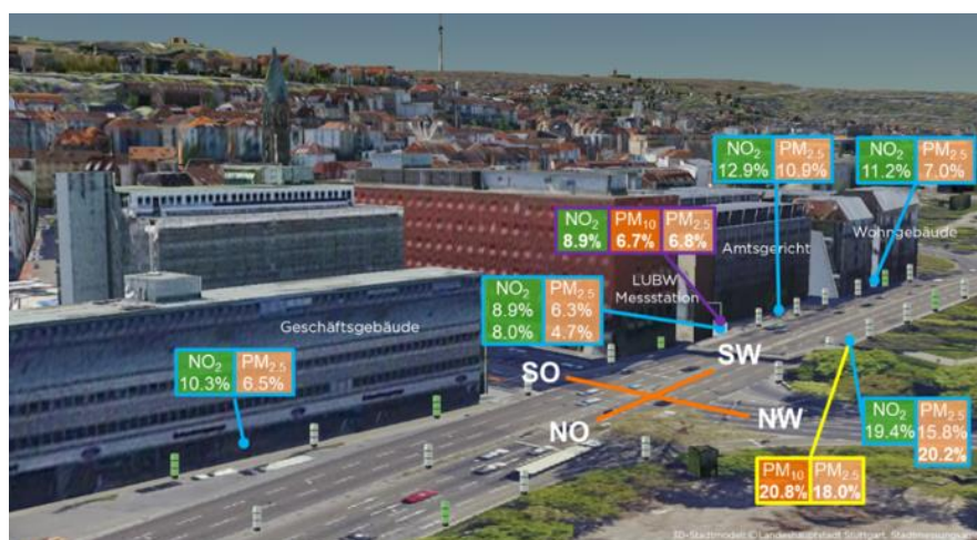
Figure 6.2 – Reduction effect at the various measurement points for the second half hour of each switching interval. Purple: LUBW; yellow: Palas Fidas 200s; blue: Födisch FDS18/GSA19.
