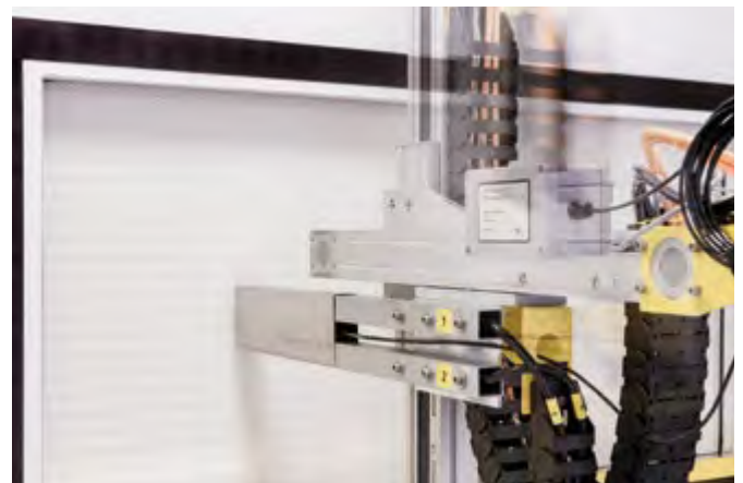
HEPA filter panel during the scan test
